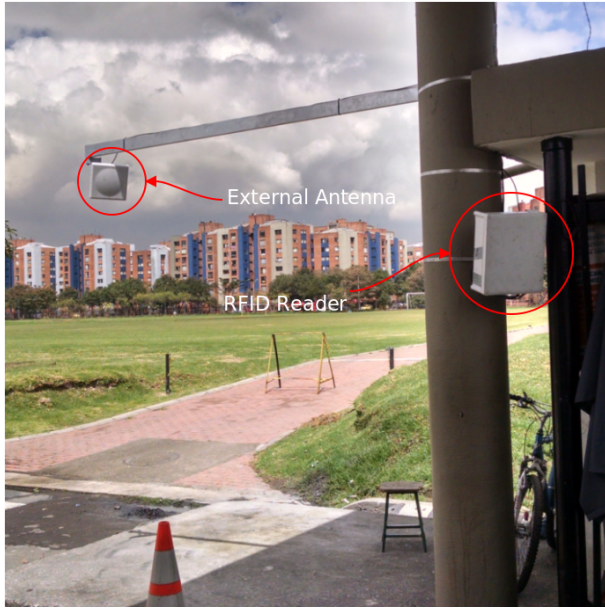
Figure 4: RFID reader installed in one of entrances of the campus. The external antenna and the RFID reader with an integrated antenna are shown.
